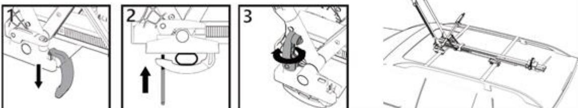
Hook the 3x brackets into the carrier (1), place the tension bolts 2x long in front and 1x short in rear, close the brackets around the carrier bars (2), loosen/tighten the quick-release levers for the desired closing force (3) and close by to fold it down.
