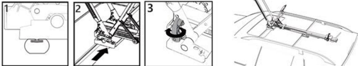
Place the T-bolts in the aluminum carrier profiles (1), slide the carrier to the desired position (2), loosen/tighten the quick-release levers for the desired closing force (3) and close by folding it down.
