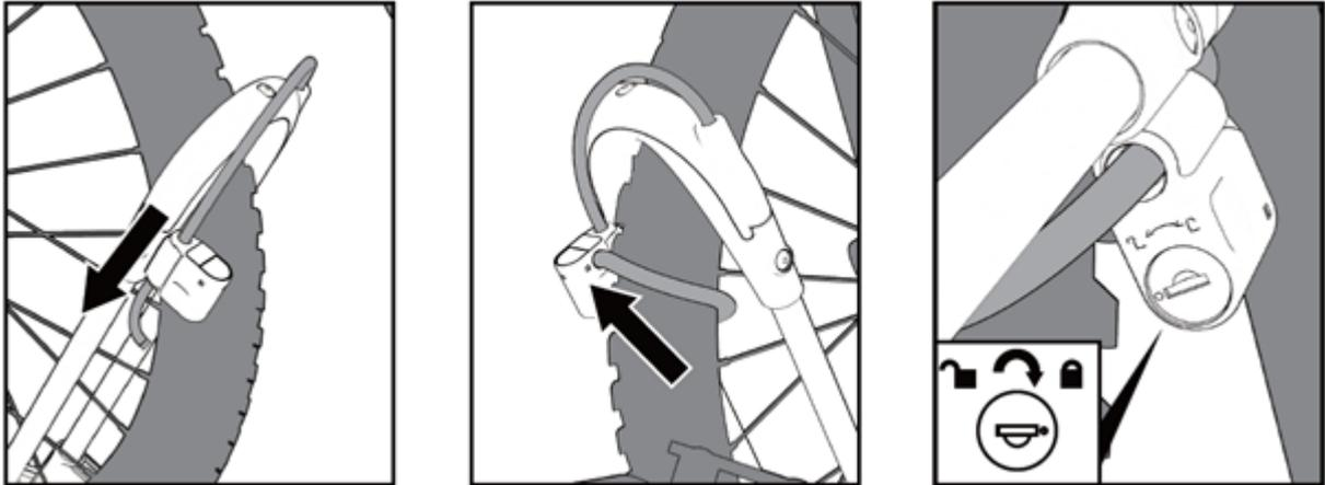
Pull the cable completely out of the front wheel support, secure it in and loop around the frame tube of the bicycle and/or through the front wheel and insert the end into the freely slidable lock housing with lock cylinder. Lock the lock cylinder to delay theft. Keep the key carefully.
